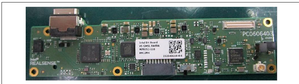
Figure 7-2 RealSense™ Vision Processor D4 Board V5
