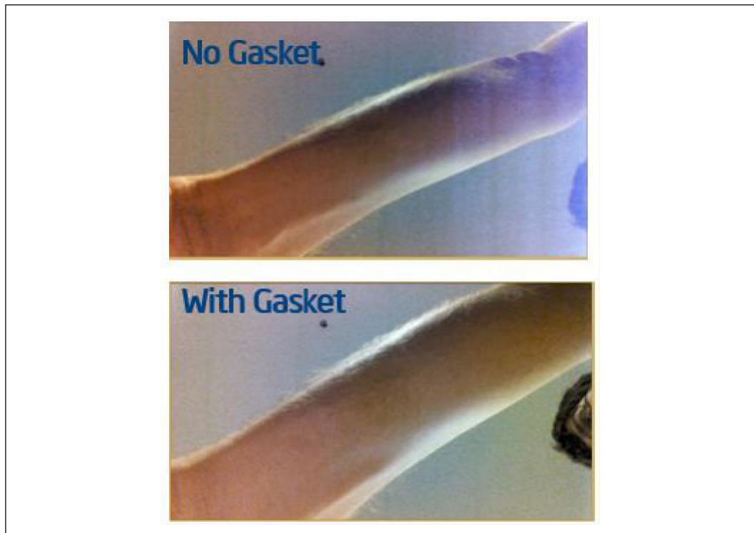
Figure 7-9 Example of Light Leakage Effects
