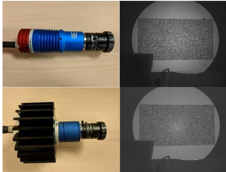
Figure 11. High power LED-based external projectors (L) and corresponding projected patterns (R). 3W model (top) and 10W (bottom).
