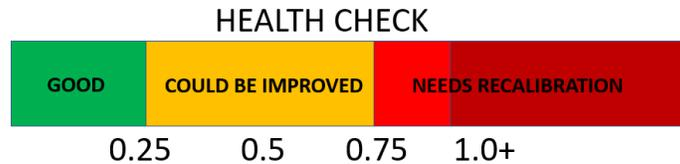
**Table 1.** The “Health-Check” indicator will return a measure of the need for recalibration. While units are operational for values below 1, it is optimal to have an absolute value below 0.25. This health-check does not need any special target.
