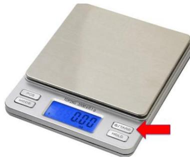
Figure 9. The “Tare” function is commonly used to remove bias and reset to a known value. When weighing objects, this means it is possible to place a bowl on a scale, “tare” to set to zero, and now measure the true weight of its contents.
