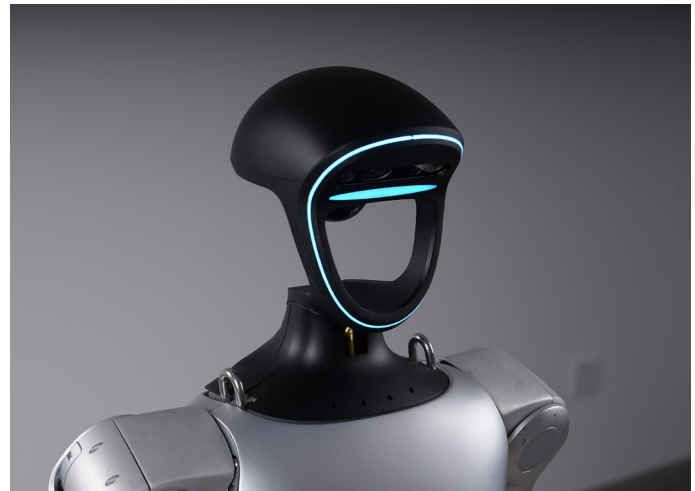
Close-up of the sensor-equipped head, enabling 3D perception for navigation and interaction.
