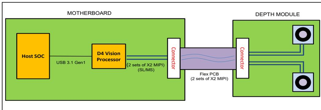
Figure 8-2. Vision Processor D4 with MIPI Host Interface
