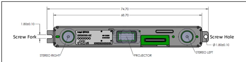
Figure 7-12. Stereo Depth Module Screw Mounting/End Mounting – D430
