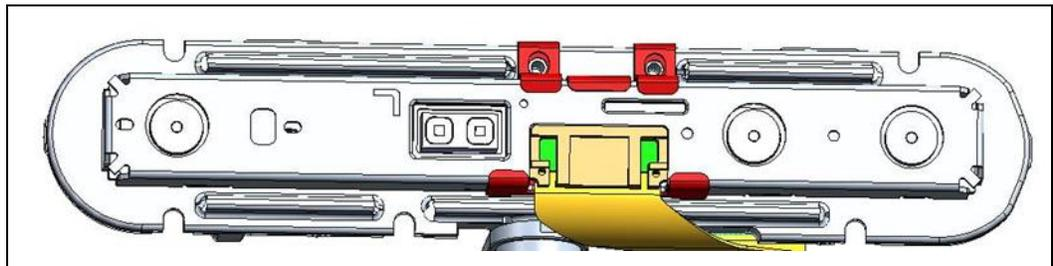
Figure 7-15. Stereo Depth Module Mid-Mounting – D401
