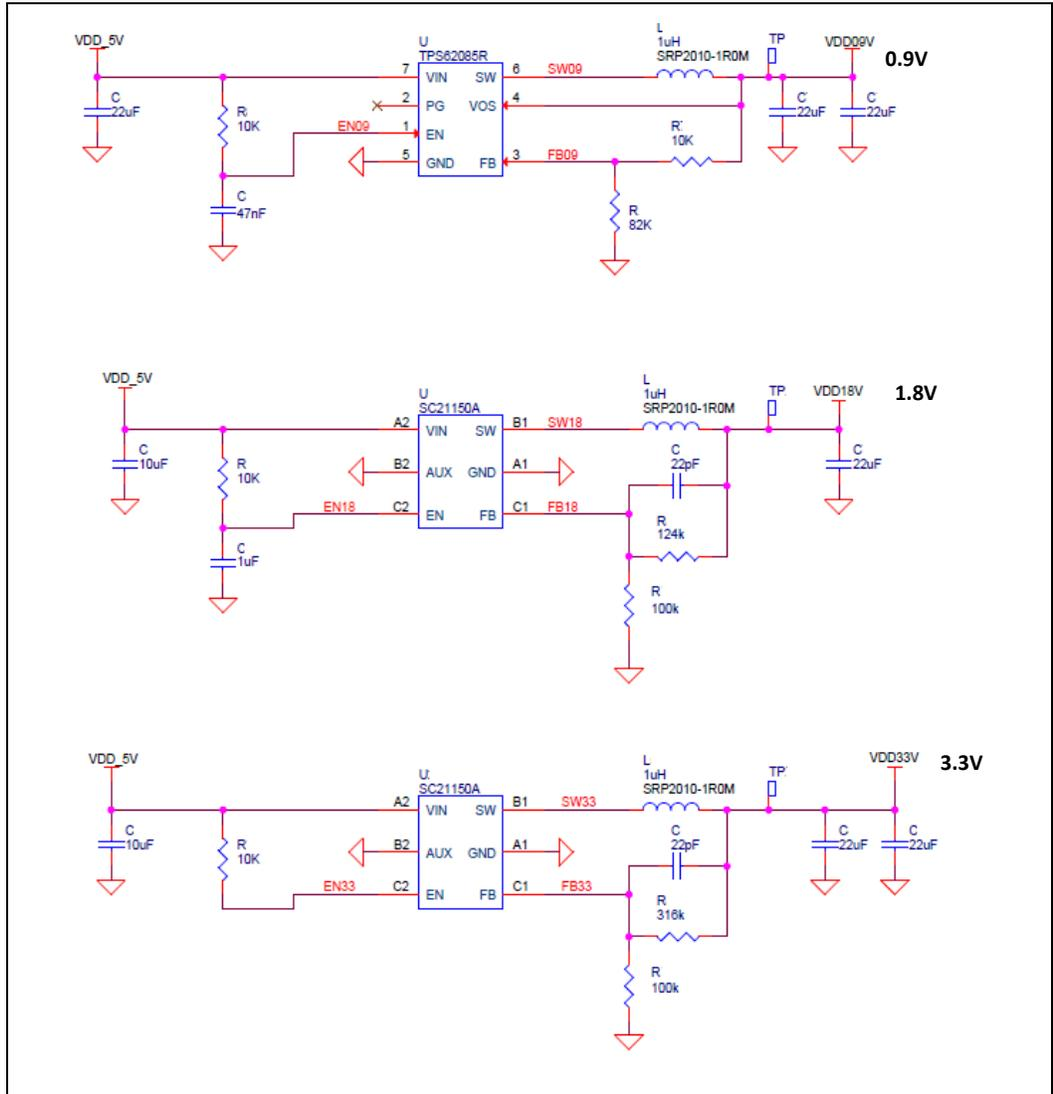
Figure 12-4. Vision Processor D4 VDD\_PG and AVDD Reference Platform Schematic
