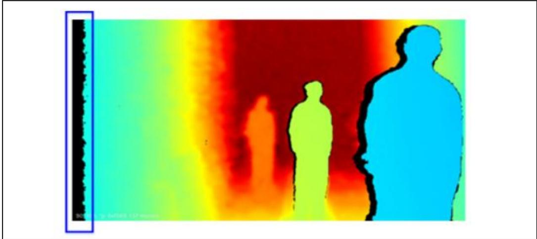
The width of the invalid depth band can be calculated using the following equations:
