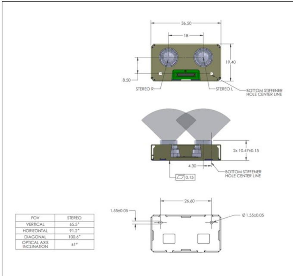
Figure 10-7. Vision Processor D4 Board USB Micro-B (RealSense™ Vision Processor D4 Board – V4)
