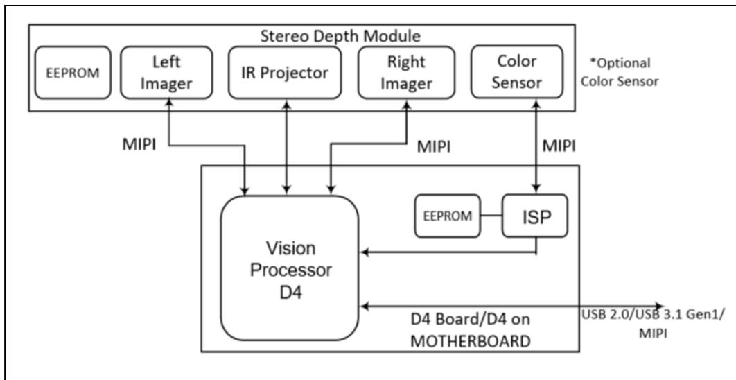
Figure 7-2. System Block Diagram – D405
