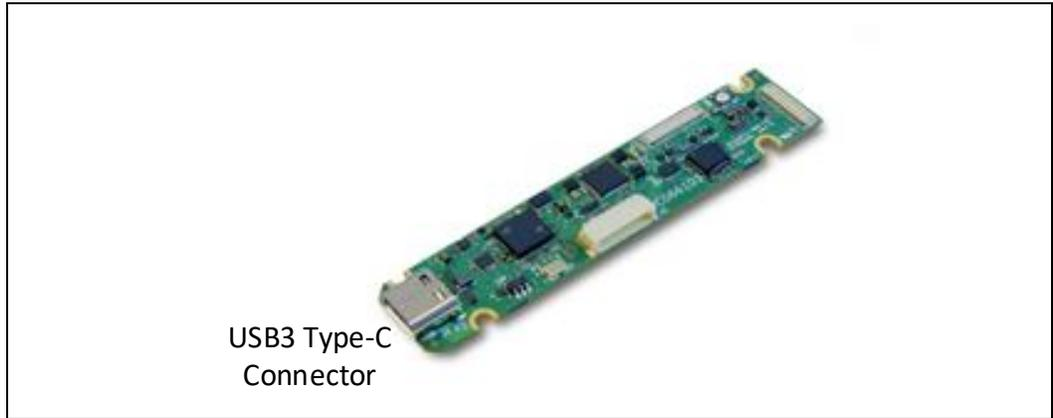
Figure 7-4. RealSense™ Vision Processor D4 Board – V4
