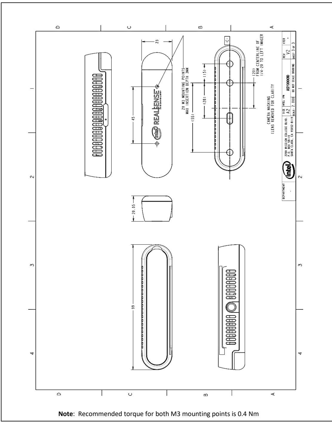
**Note:** Recommended torque for both M3 mounting points is 0.4 Nm
