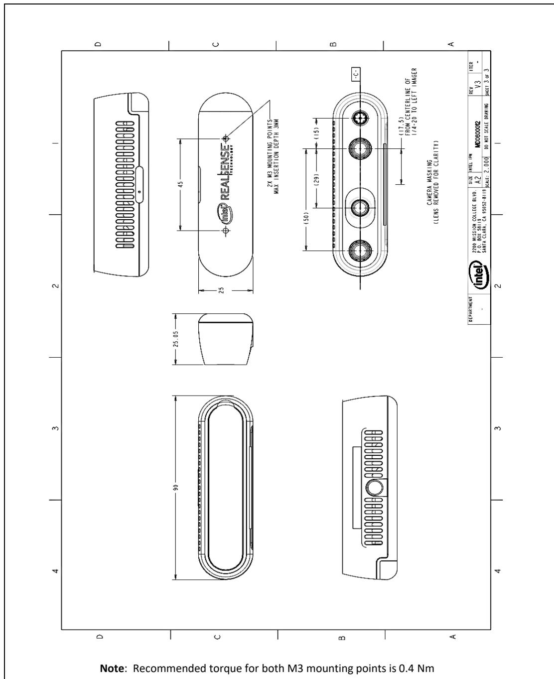
Figure 10-10. RealSense™ Depth Camera D435f/D435if NIR Filter
