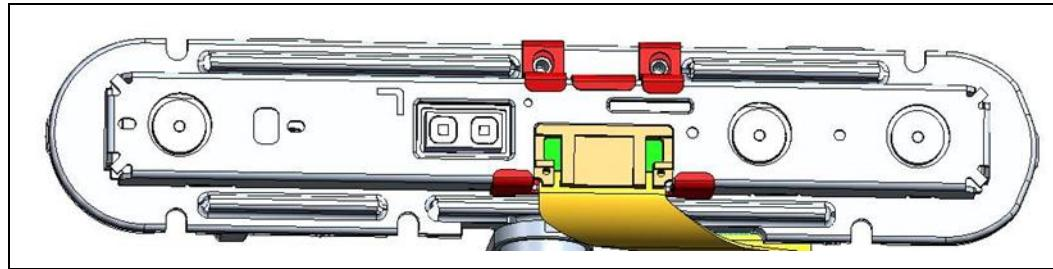
**Figure 7-15. Stereo Depth Module Mid-Mounting – D401**
