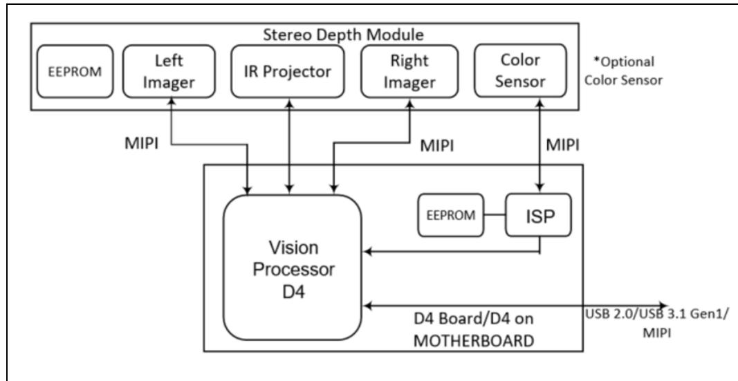
**Figure 7-2. System Block Diagram – D405**
