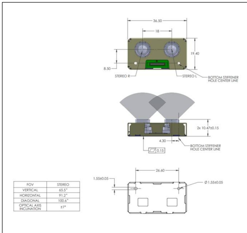
Figure 10-6. Vision Processor D4 Board USB Type-C (RealSense™ Vision Processor D4 Board – V1 and V3)
