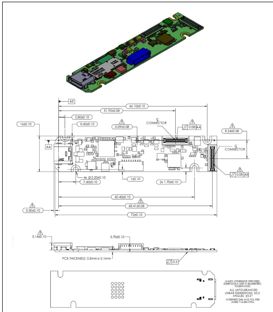
**Figure 10-7. Vision Processor D4 Board USB Micro-B (RealSense™ Vision Processor D4 Board – V4)**
