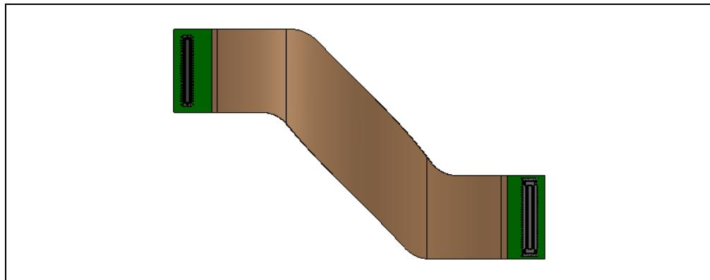
Figure 3-12. Rigid Interposer – D415, D435, D435i, D435f, D435if, D455, D455f, D456 (Illustration)
