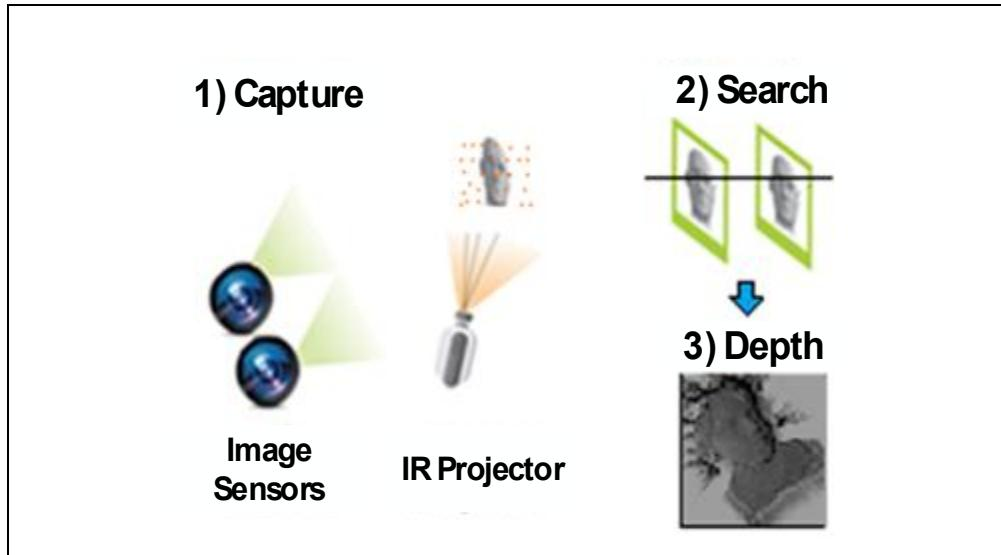
The depth pixel value is a measurement from the parallel plane of the imagers and not the absolute range as illustrated.
