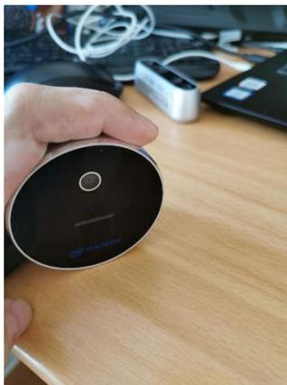
**Figure 4-8 L515 Position #1 (Upright facing out position)**
