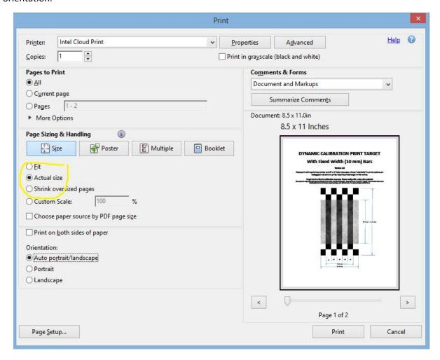
The physical image after printed should be 68.4 mm wide and 121.6 mm high - same as iPhone 7 plus 5.5" display. The 5 vertical bars in the middle (3 black and 2 white) in equal spacing, each 10 mm wide. The vertical bar length is 100.0 mm, as illustrated around the target image.
