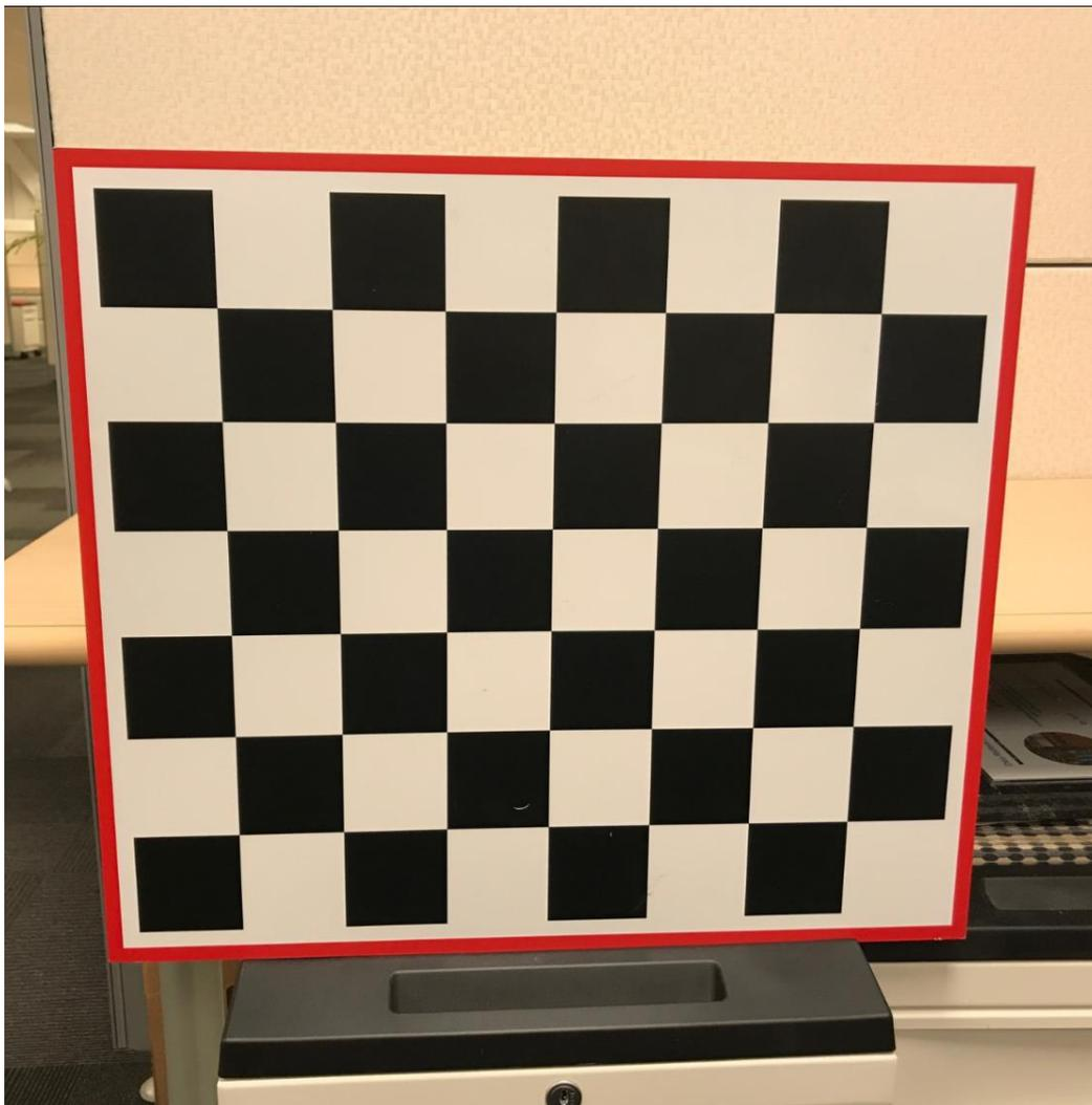
**Figure 3-3 8x7 60x60 mm Checker Calibration Target**
