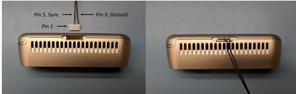
If the distance between cameras is relatively small, less than approximately 3 meters, passive interconnect is suitable. An example circuit with ESD protection is shown below. Shielded twisted pair cable is preferred. The shield can be connected to ground (pin 9) at the master camera connector and left unconnected at other connectors.
