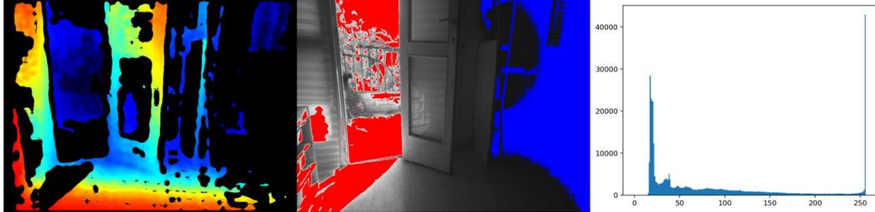
**Figure 14. Mixed indoor and outdoor scene. Left: Depth map , Middle: Left monochrome image with inpainting to show saturation (red) and underexposed (blue) regions. . Right: left image brightness histogram, showing the the bi-modal distribution of high and low exposure.**
