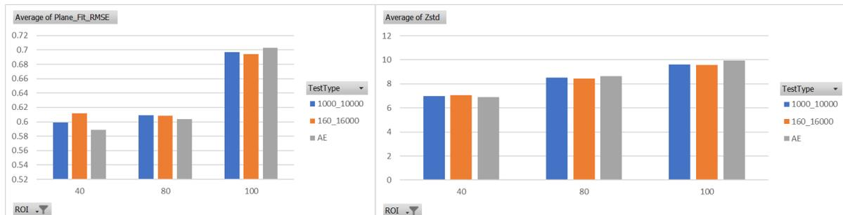
Figure 19. Plane fit RMSE and Z-std metrics for indoor lab scene. The blue bar is with HDR exposure of (1ms & 10ms). The red bar is with auto exposure of (0.16ms & 16ms), while the grey bar is the simple single frame auto-exposure. The y-axis is the error in mm. Smaller is better. We see no significant change across these KPIs. The x-axis is the distance away from the object in mm.
