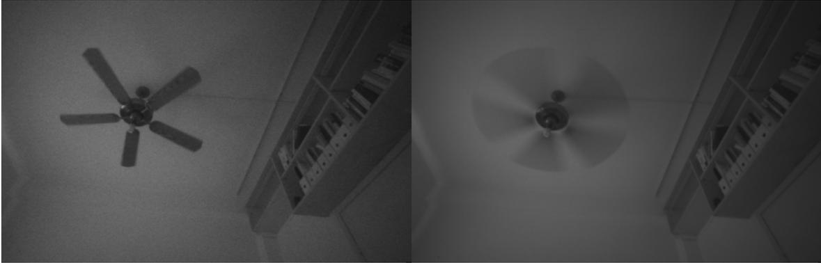
Figure 4. Same scene captured with high gain and short exposure (left) vs low gain and longer exposure (right). This scene was captured with the global shutter imagers of the D435, so there are no additional rolling shutter artefacts of the fan.
