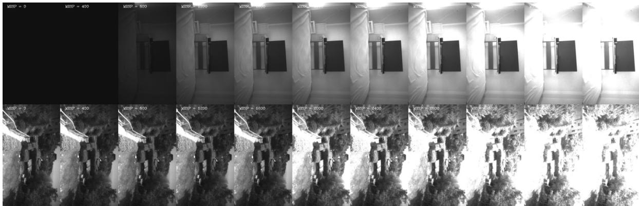
**Figure 7. Effect of adjusting auto-exposure set-point for an indoor (top) and outdoor (bottom) scene. The setpoint is increased going from left side images to right-side images. Note that in the outdoor scene the image cannot get any darker on the left, due to sensor minimal exposure limitations.**
