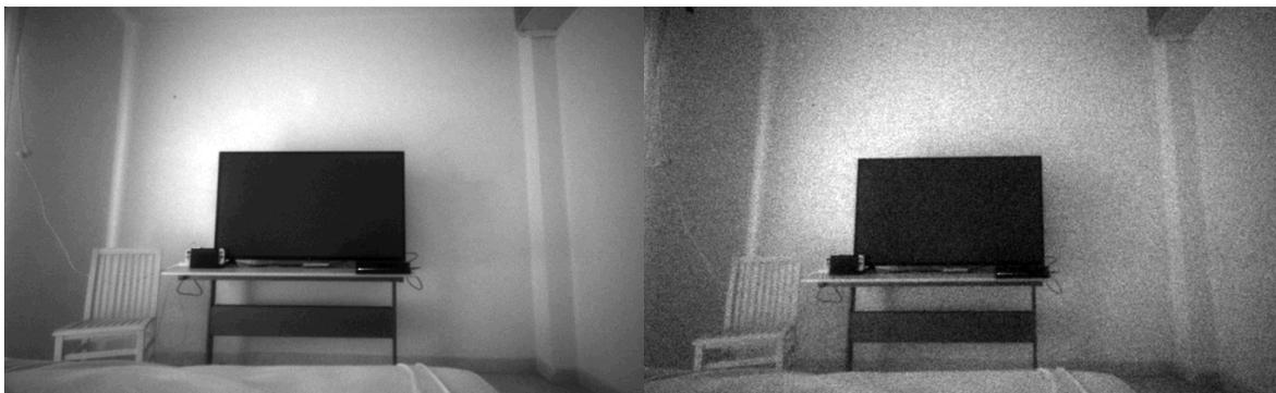
**Figure 3. Similar level of brightness achieved by adjusting the exposure (left) vs adjusting gain (right)**
