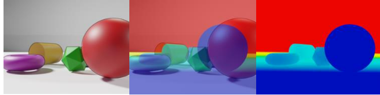
Figure 9. View from the color camera (left), view from the depth sensor (right), color and depth frames overlaid on top of each other (middle)
